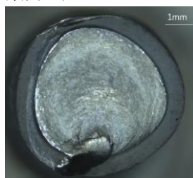
扭转断裂螺栓
